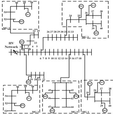
Fig. 2: IEEE-33 bus based test system
